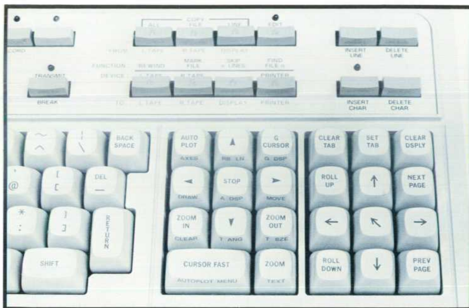
Fig. 2. Graphics control group replaces the numeric keypad of other 2640 terminals. Each graphics key has two functions. The function on the front of the key is accessed by pressing the SHIFT key and the graphics key simultaneously. The keys at right control the alphanumeric display.
