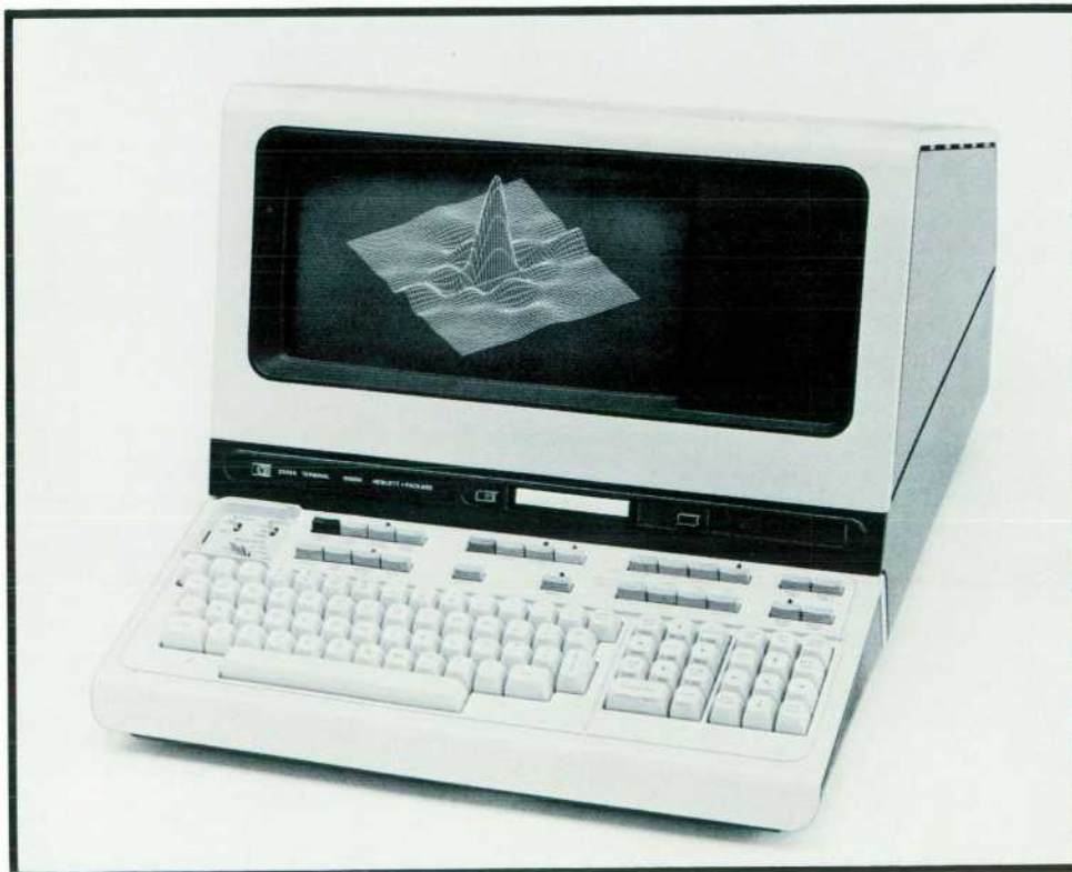
Fig. 1. Model 2648A Graphics Terminal has both graphics and alphanumeric capabilities. Raster scan technology provides such features as area shading, selective erase, and compatibility with matrix printers. A comprehensive self test verifies operation and helps identify the defective module or component.
